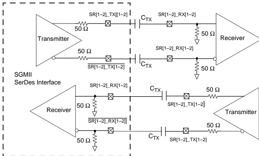
Figure 39. 4-Wire AC-Coupled SGMII Serial Link Connection Example
