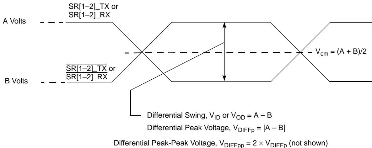
**Figure 4. Differential Voltage Definitions for Transmitter or Receiver**
