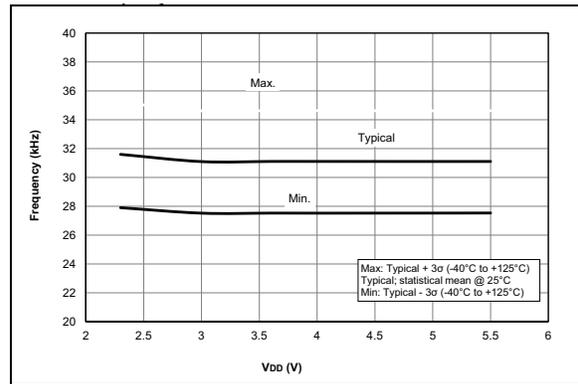
**FIGURE 32-58:** LFINTOSC Frequency, PIC16LF1788/9 Only.
