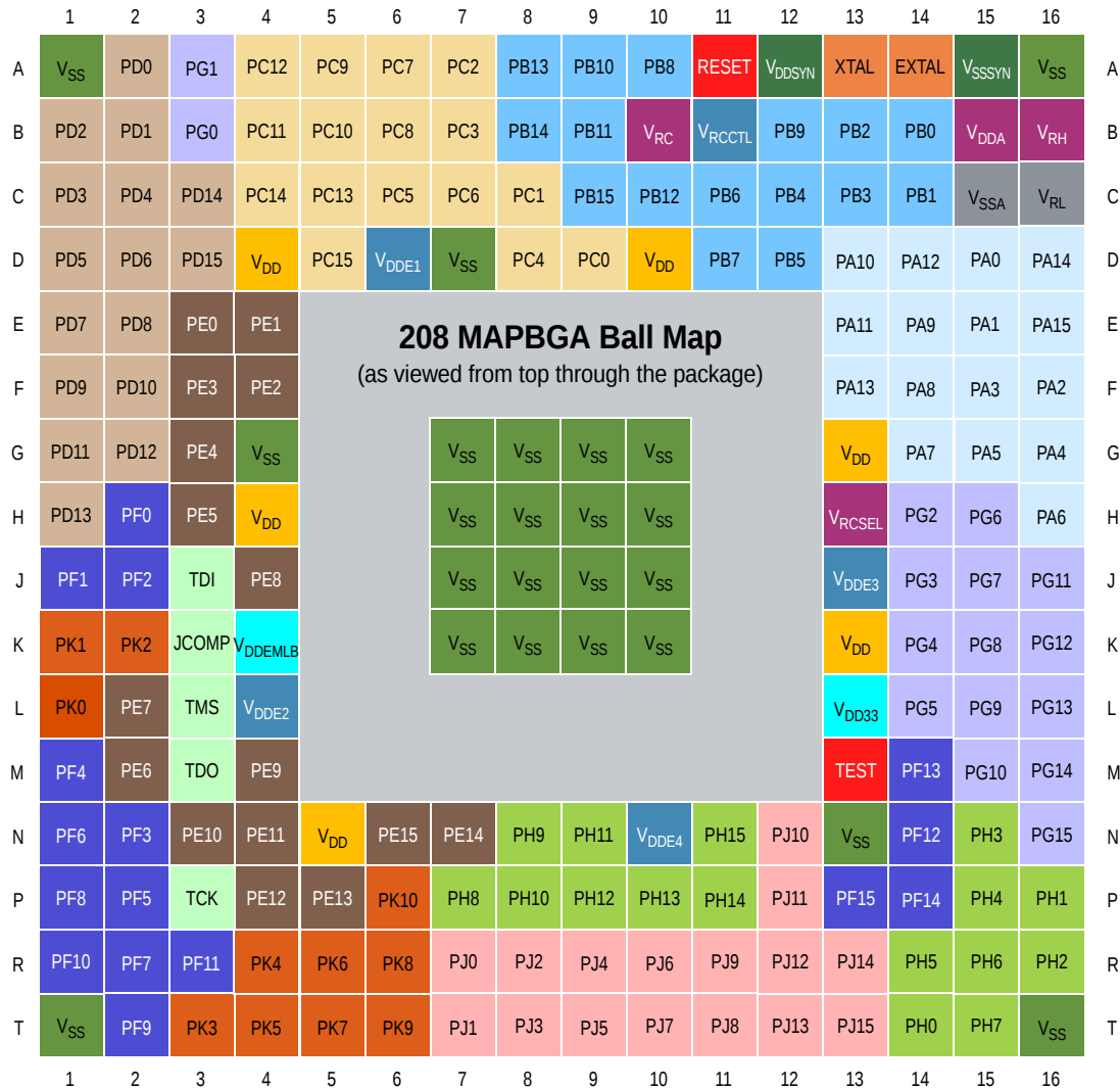
Figure 3. MPC5668x 208-ball MAPBGA (full diagram)
