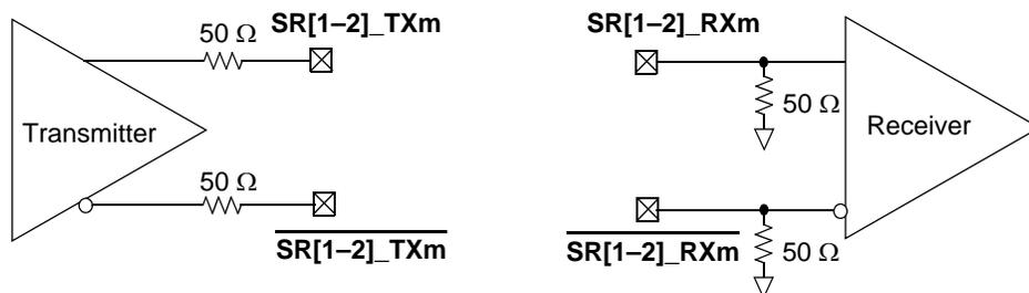
**Note:** The [1–2] indicates the specific SerDes Interface (1 or 2) and the m indicates the specific channel within that interface (0,1,2,3). Actual signals are assigned by the HRCW assignments at reset (see **Chapter 5, Reset** in the reference manual for details)
