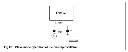
In slave mode the input clock signal should be coupled by means of a capacitor of 100 pF (Figure 28), with an amplitude between 200 mV(RMS) and 1000 mV(RMS). This corresponds to a square wave signal with a signal swing of between 280 mV and 1.4 V. The XTALOUT pin in this configuration can be left unconnected.
