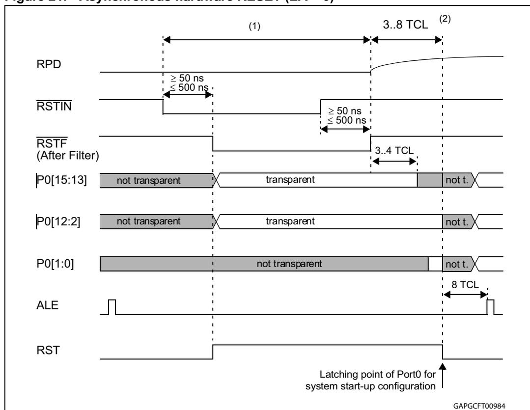
1. Longer than Port0 settling time + PLL synchronization (if needed, that is P0(15:13) changed). Longer than 500ns to take into account of Input Filter on RSTIN pin.
