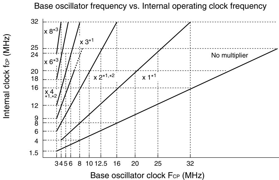
\*1 : When the PLL multiplier is  $\times 1$ ,  $\times 2$ ,  $\times 3$  or  $\times 4$  and the internal clock is  $20 \text{ MHz} < f_{\text{CP}} \leq 32 \text{ MHz}$ , set DIV2 bit = “1”\*4, CS2 bit = “1” in the PSCCR register.
