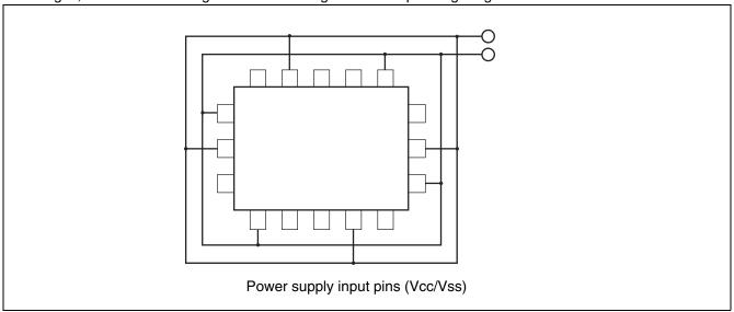
In addition, care must be given to connecting the VCC and VSS pins of this device to the current supply source with as low impedance as possible. It is recommended that a 1.0  $\mu$ F bypass capacitor be connected between the VCC and VSS pins as close to the pins as possible.
