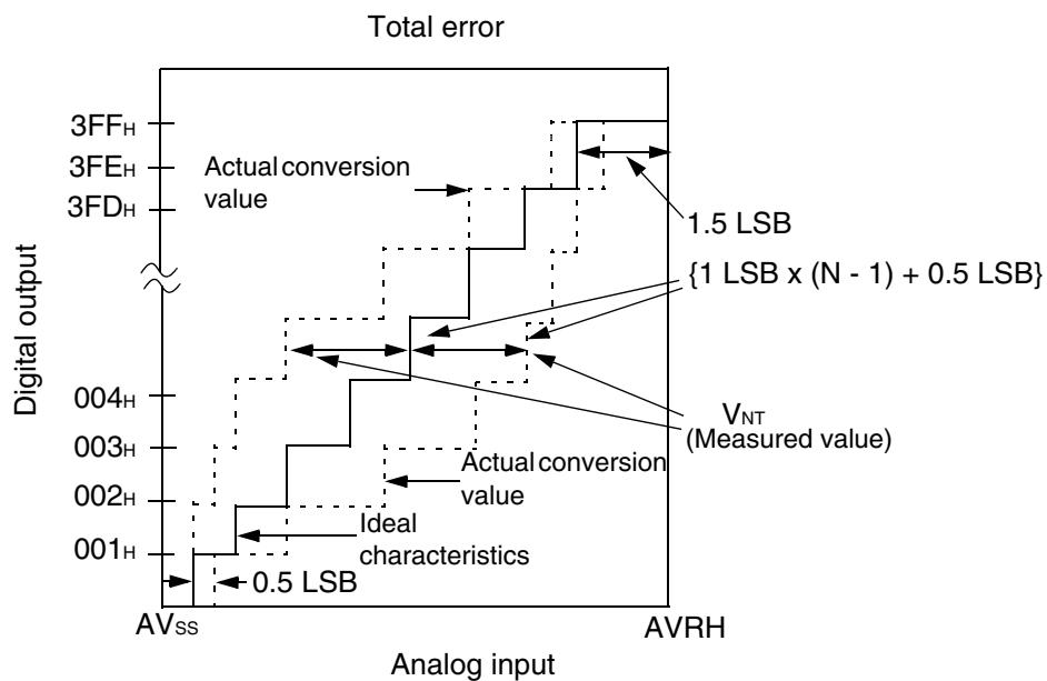
$$\text{Total error for digital output } N = \frac{V_{NT} - \{1 \text{ LSB} \times (N - 1) + 0.5 \text{ LSB}\}}{1 \text{ LSB}} \text{ [LSB]}$$
