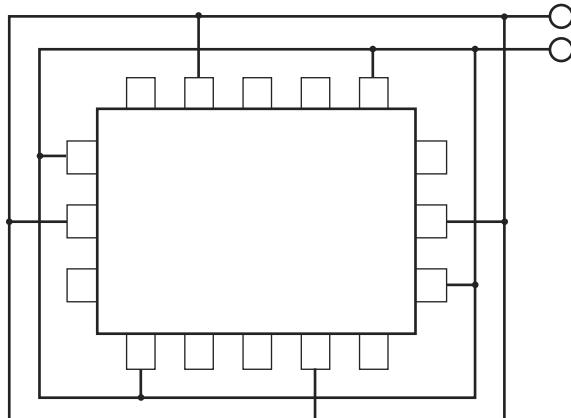
Power supply input pins (Vcc/Vss)
