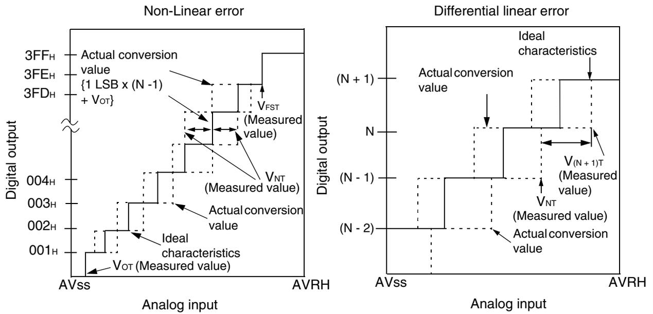
$$\text{Non-linear error of digital output } N = \frac{V_{NT} - \{1 \text{ LSB} \times (N - 1) + V_{OT}\}}{1 \text{ LSB}} \text{ [LSB]}$$
