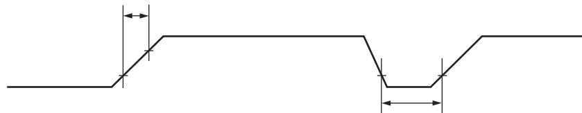
Note : Extreme variations in power supply voltage may trigger a power-on reset. When the power supply voltage is changed during operation, it is recommended that increases in the voltage smoothed out as shown in the following diagram. The PLL clock of the device should not be in use when varying the voltage. However, the PLL clock may continue to be used if the rate of the voltage drop is 1 V/s or less.
