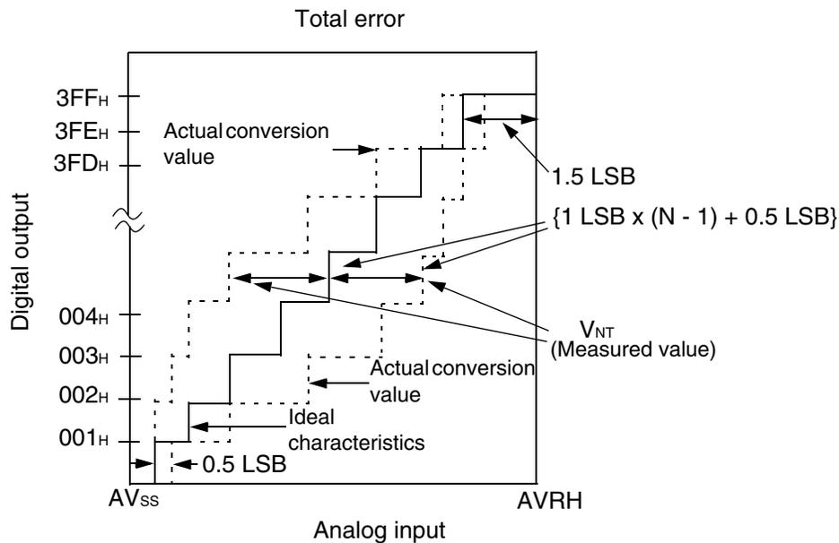
$$\text{Total error for digital output } N = \frac{V_{NT} - \{1 \text{ LSB} \times (N - 1) + 0.5 \text{ LSB}\}}{1 \text{ LSB}} \quad [\text{LSB}]$$
