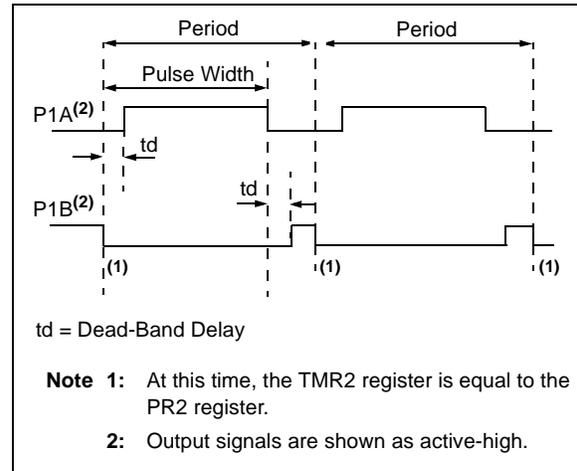
**FIGURE 11-18: EXAMPLE OF HALF-BRIDGE APPLICATIONS**
