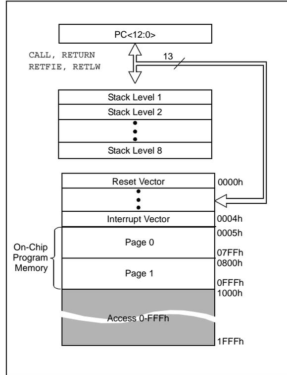
**FIGURE 2-3: PROGRAM MEMORY MAP AND STACK FOR THE PIC16F677/PIC16F687**
