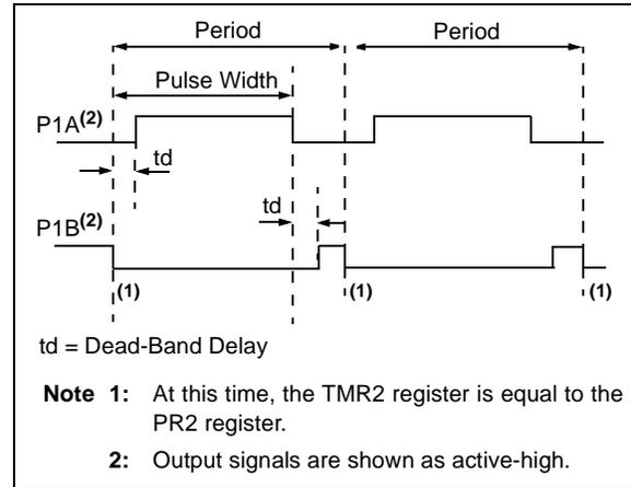
**FIGURE 11-9: EXAMPLE OF HALF-BRIDGE APPLICATIONS**
