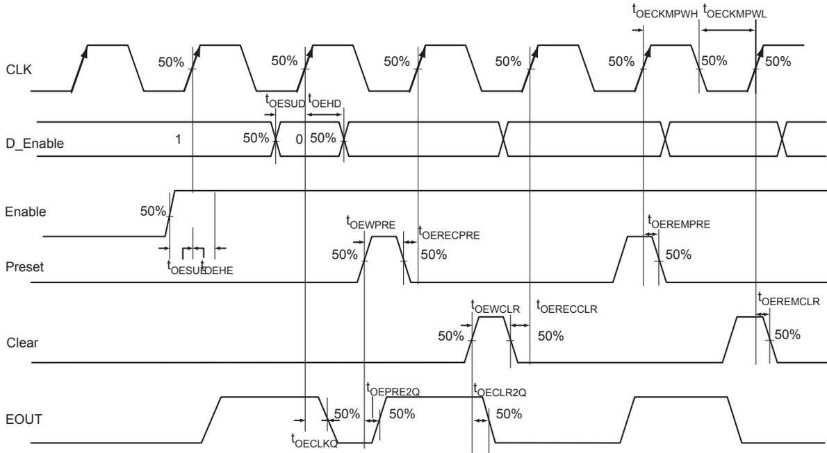
Figure 2-139 • Output Enable Register Timing Diagram
