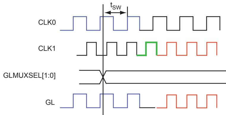
**Figure 2-26 • NGMUX Waveform**
