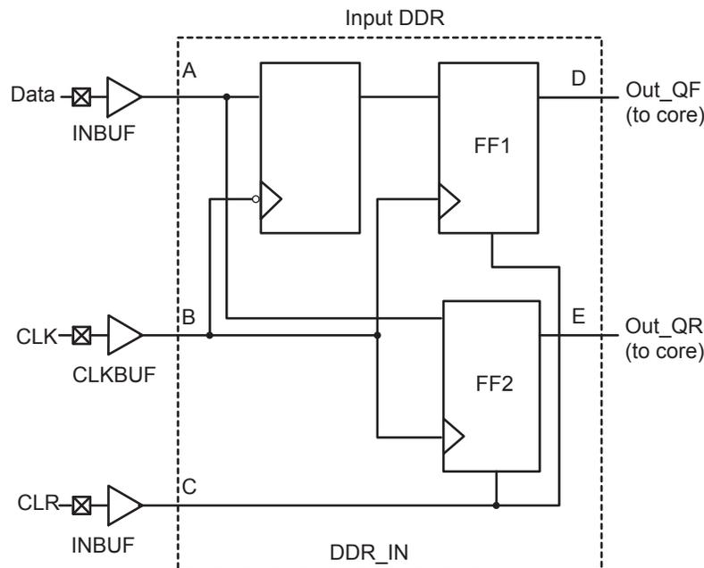
**Figure 2-100 • DDR Input Register Support in Fusion Devices**
