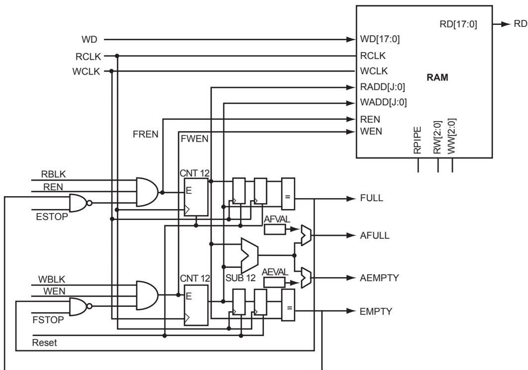
**Figure 2-47 • Fusion RAM Block with Embedded FIFO Controller**
