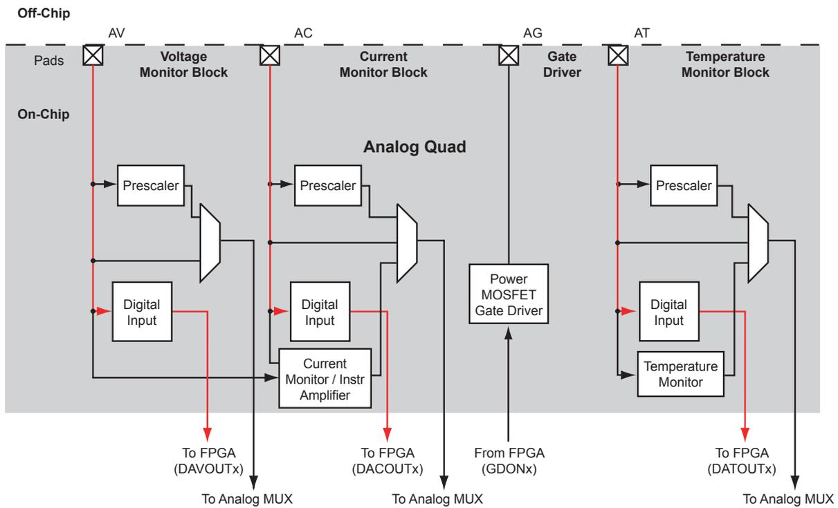
Figure 2-68 • Analog Quad Direct Digital Input Configuration
