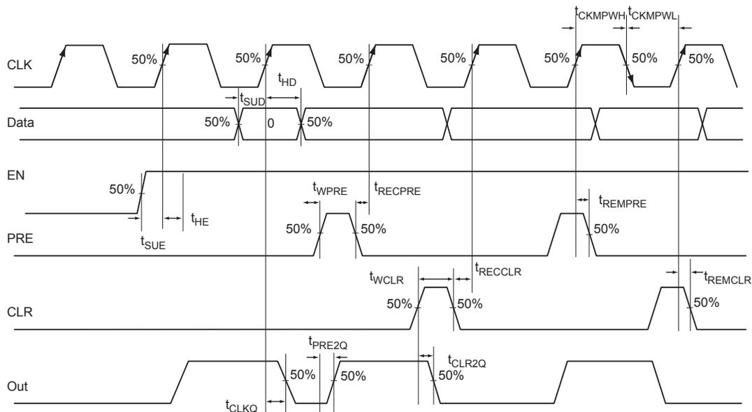
**Figure 2-6 • Sequential Timing Model and Waveforms**
