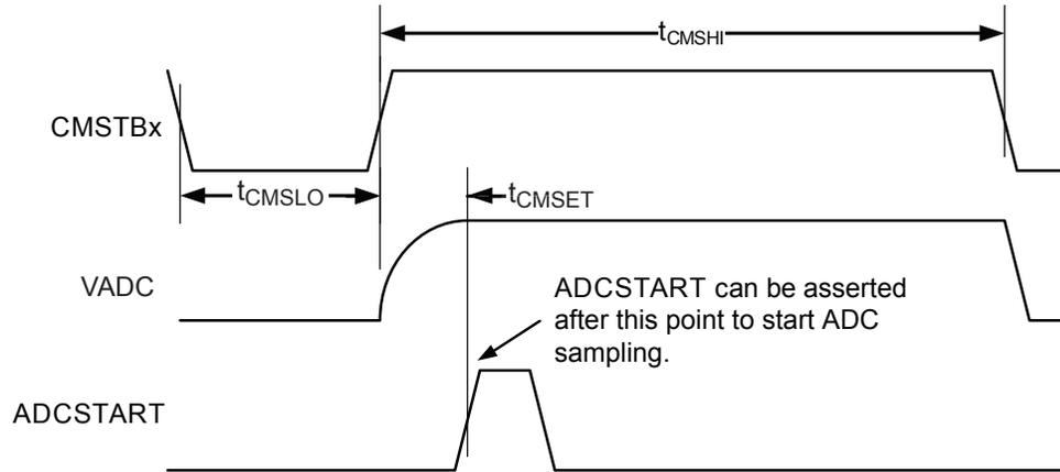
**Figure 2-70 • Timing Diagram for Current Monitor Strobe**
