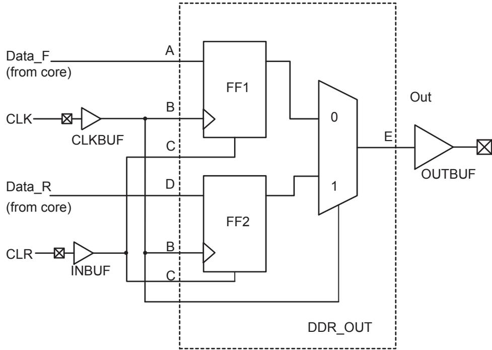
**Figure 2-101 • DDR Output Support in Fusion Devices**
