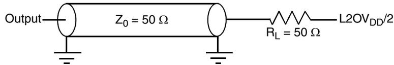
**Figure 10. AC Test Load for the L2 Interface**
