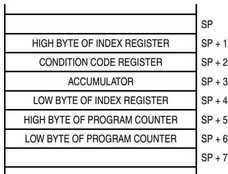
Figure 18-12. Stack Pointer at Monitor Mode Entry
