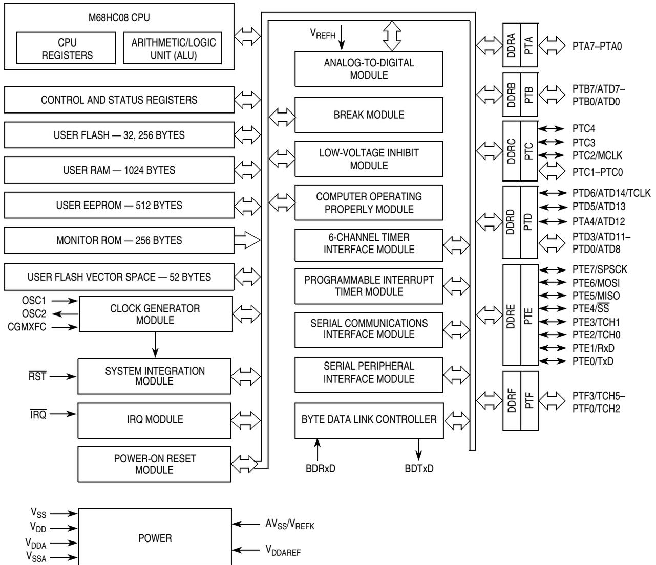
Figure 1-1. MCU Block Diagram for the MC68HC908AS32A
