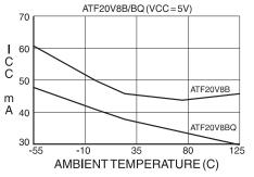
SUPPLY CURRENT vs. AMBIENT TEMPERATURE
