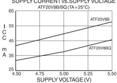
SUPPLY CURRENT vs. SUPPLY VOLTAGE
