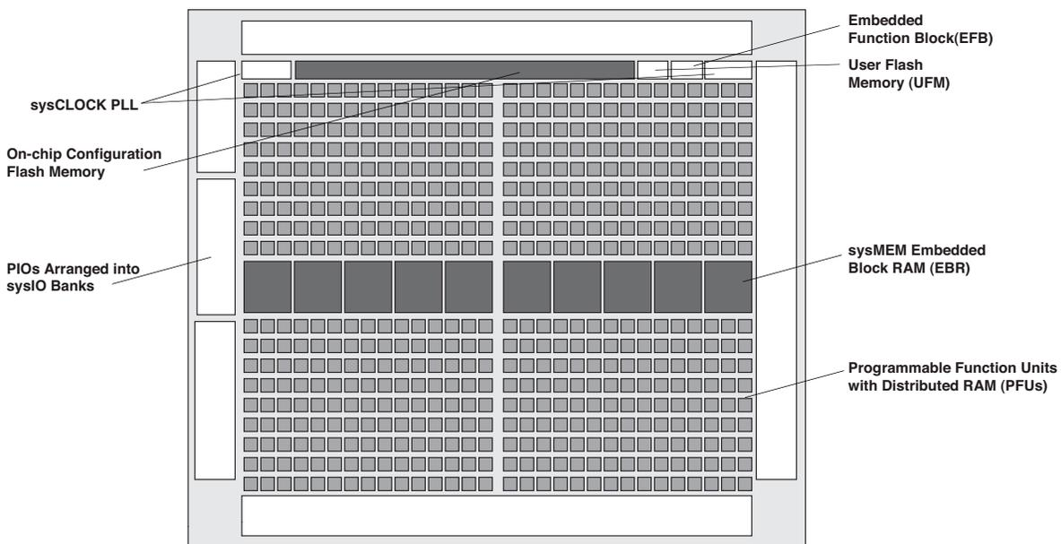
Note: MachXO2-1200U, MachXO2-2000/U and MachXO2-7000 are similar to MachXO2-4000. MachXO2-1200U and MachXO2-2000 have a lower LUT count, one PLL, and eight EBR blocks. MachXO2-2000U has a lower LUT count, two PLLs, and 10 EBR blocks. MachXO2-7000 has a higher LUT count, two PLLs, and 26 EBR blocks.
