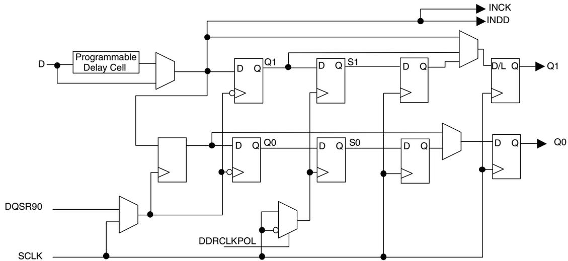
Figure 2-17. Output Gearbox
