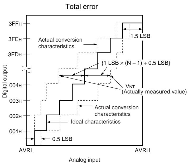
$$\text{Total error of digital output "N"} = \frac{V_{NT} - \{1 \text{ LSB} \times (N - 1) + 0.5 \text{ LSB}\}}{1 \text{ LSB}} \text{ [LSB]}$$
