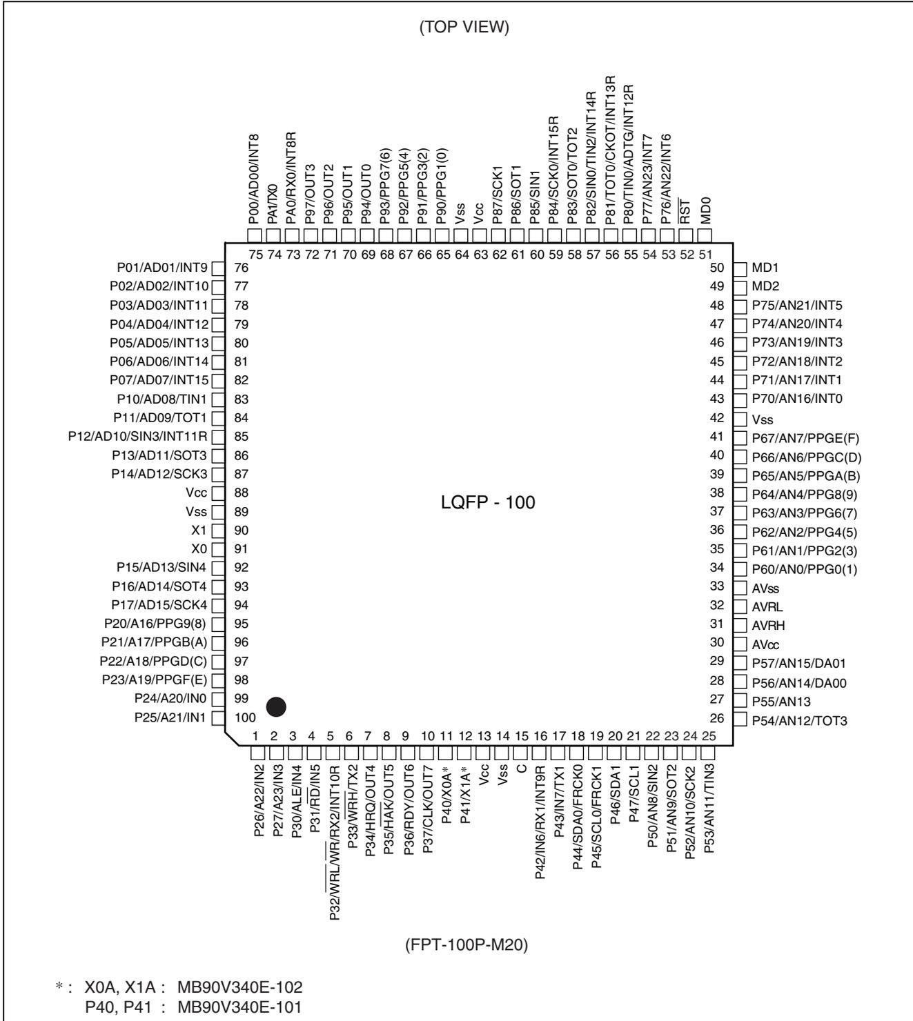
This pin assignment is for using MB90V340E-101/102 via probecable as MB90340E.
