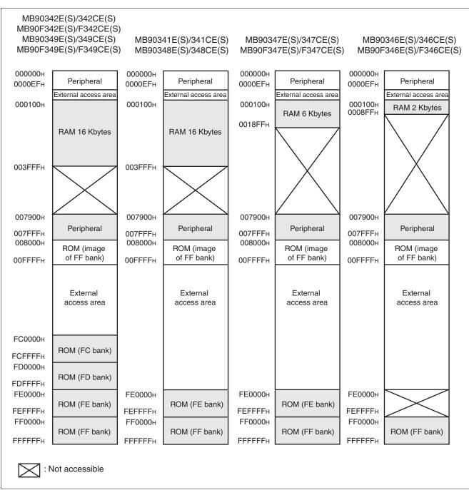
Note: :An image of the data in the FF bank of ROM is visible in the upper part of bank 00, which makes it possible for the C compiler to use the small memory model. The lower 16 bits of addresses in the FF bank are the same as the lower 16 bits of addresses in the 00 bank so that tables stored in the ROM can be accessed without using the far specifier in the pointer declaration.
