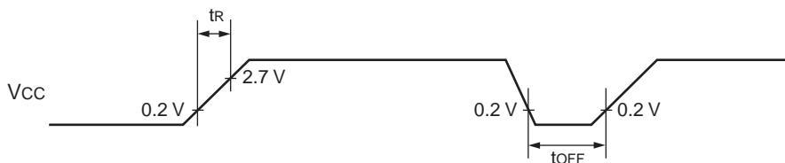
**Note:** : If you change the power supply voltage too rapidly, a power on reset may occur. We recommend that you startup smoothly by restraining voltages when changing the power supply voltage during operation, as shown in the figure below. Perform while not using the PLL clock. However, if voltage drops are within 1 V/s, you can operate while using the PLL clock.
