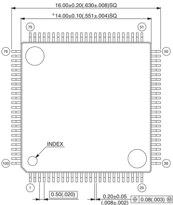
Note 1) \* : These dimensions do not include resin protrusion.
