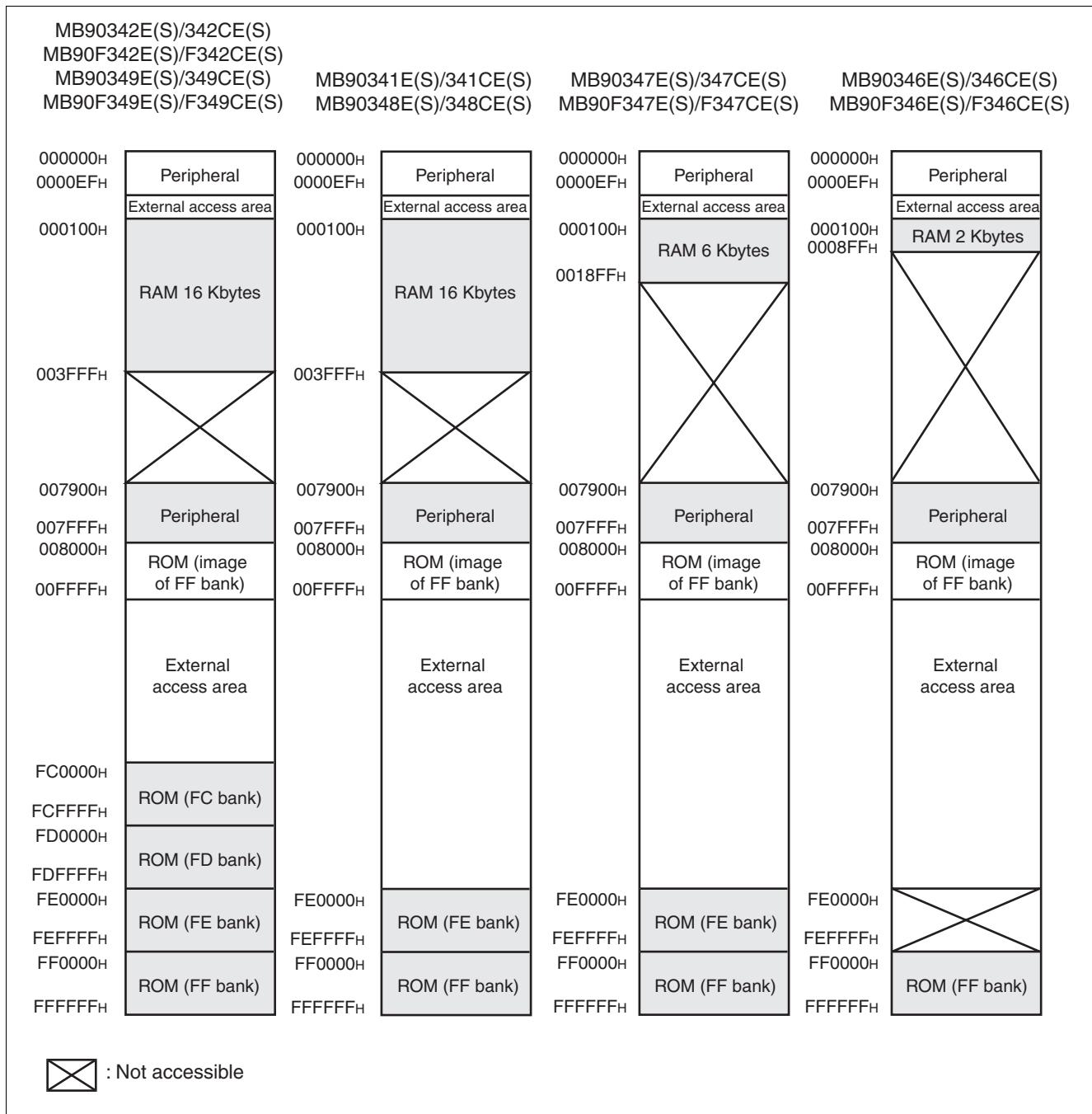
**Note:** An image of the data in the FF bank of ROM is visible in the upper part of bank 00, which makes it possible for the C compiler to use the small memory model. The lower 16 bits of addresses in the FF bank are the same as the lower 16 bits of addresses in the 00 bank so that tables stored in the ROM can be accessed without using the far specifier in the pointer declaration.
