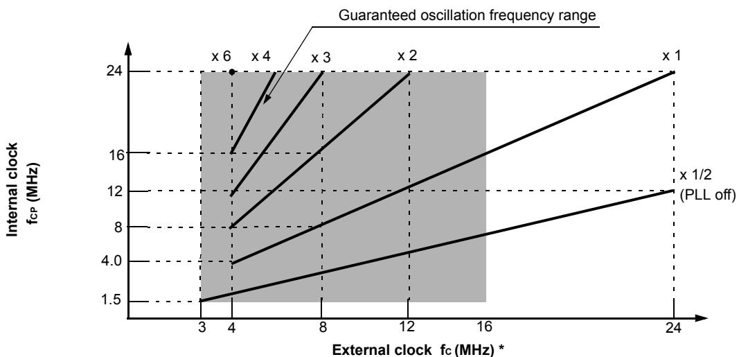
\* : When using a crystal oscillator or ceramic oscillator, the maximum oscillation clock frequency is 16 MHz
