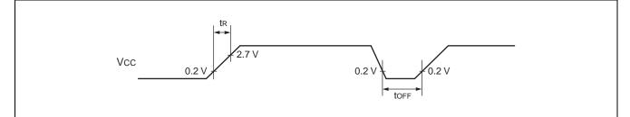
**Note:** : If you change the power supply voltage too rapidly, a power on reset may occur. We recommend that you startup smoothly by restraining voltages when changing the power supply voltage during operation, as shown in the figure below. Perform while not using the PLL clock. However, if voltage drops are within 1 V/s, you can operate while using the PLL clock.
