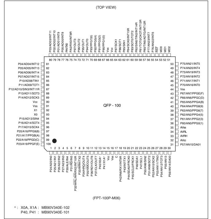
This pin assignment is for using MB90V340E-101/102 via probecable as MB90340E.
