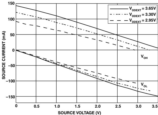
Figure 30. Drive Current A (High  $V_{DDEXT}$ )
