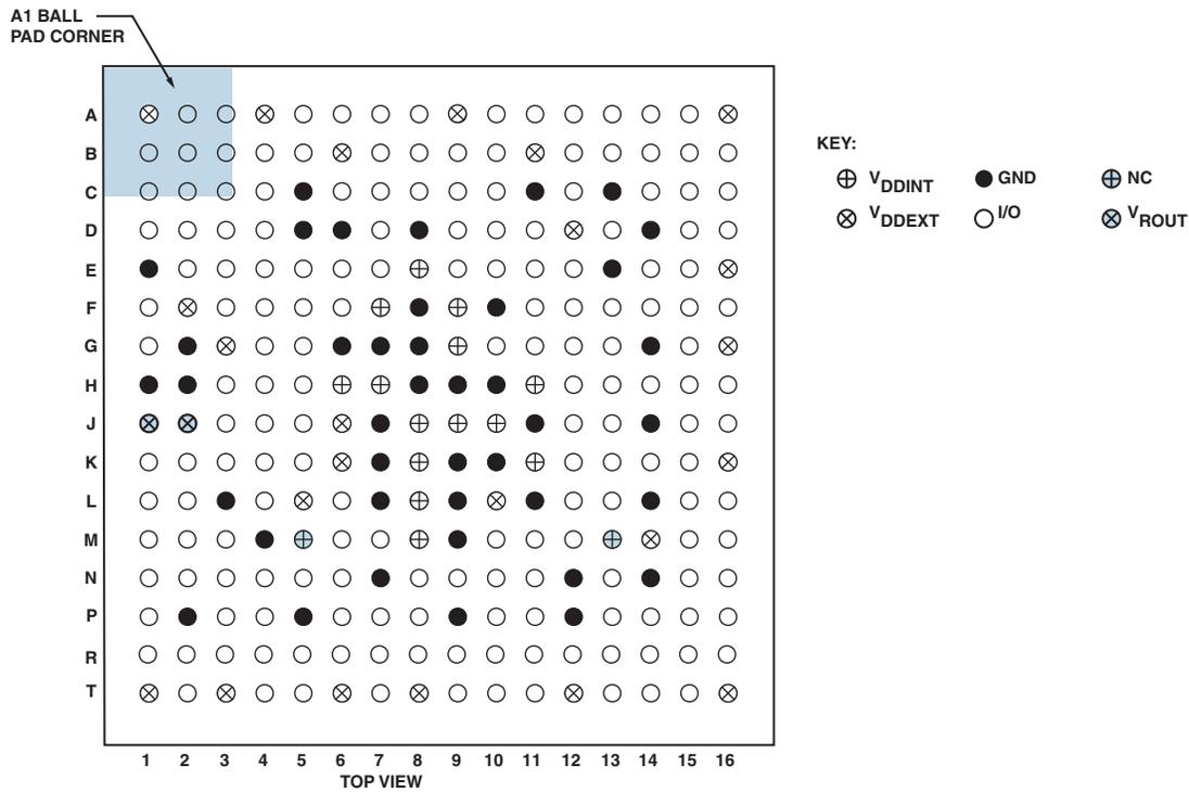
Figure 50. 256-Ball CSP\_BGA Ball Configuration (Top View)
