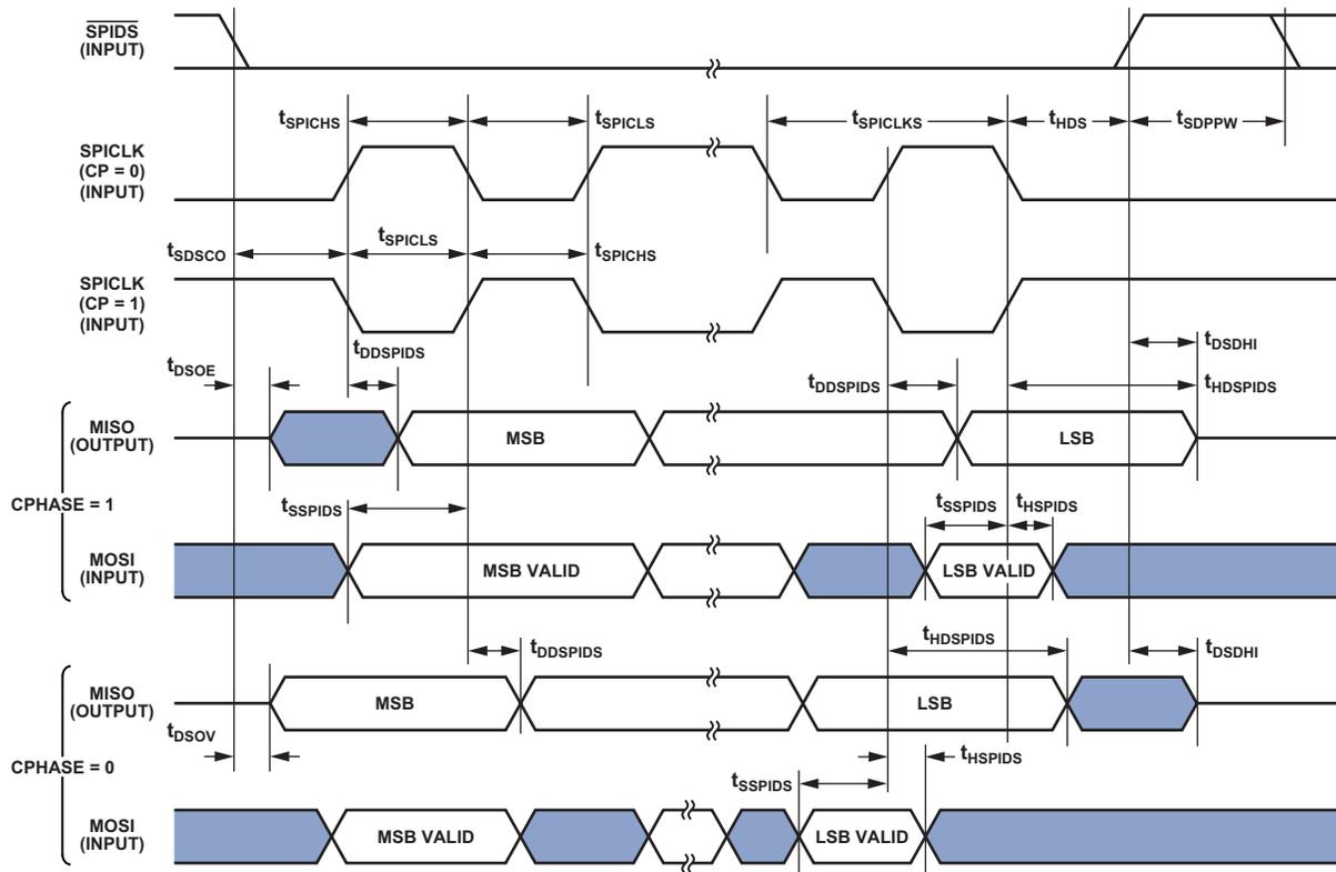
Figure 24. Serial Peripheral Interface (SPI) Port—Slave Timing
