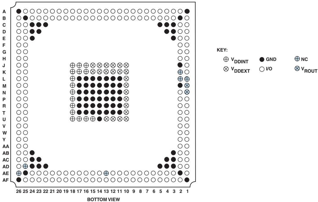
Figure 53. 297-Ball PBGA Ball Configuration (Bottom View)
