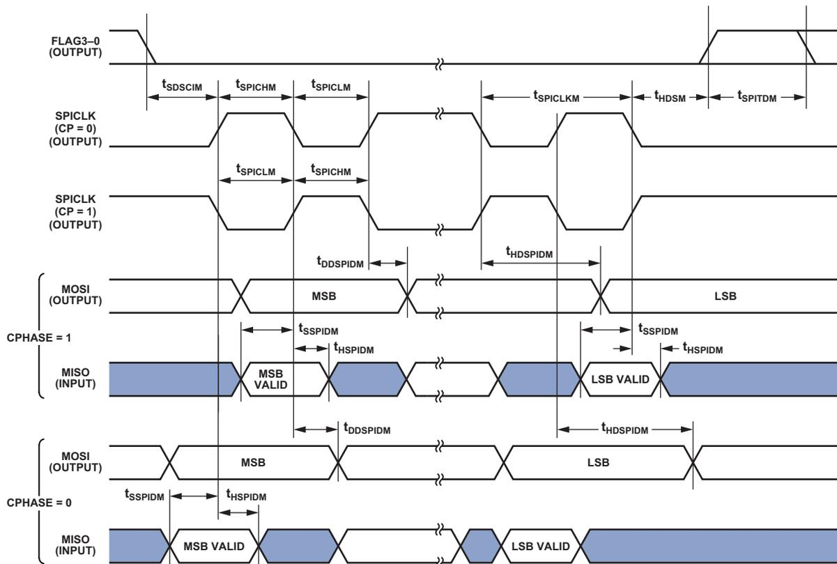
Figure 23. Serial Peripheral Interface (SPI) Port—Master Timing
