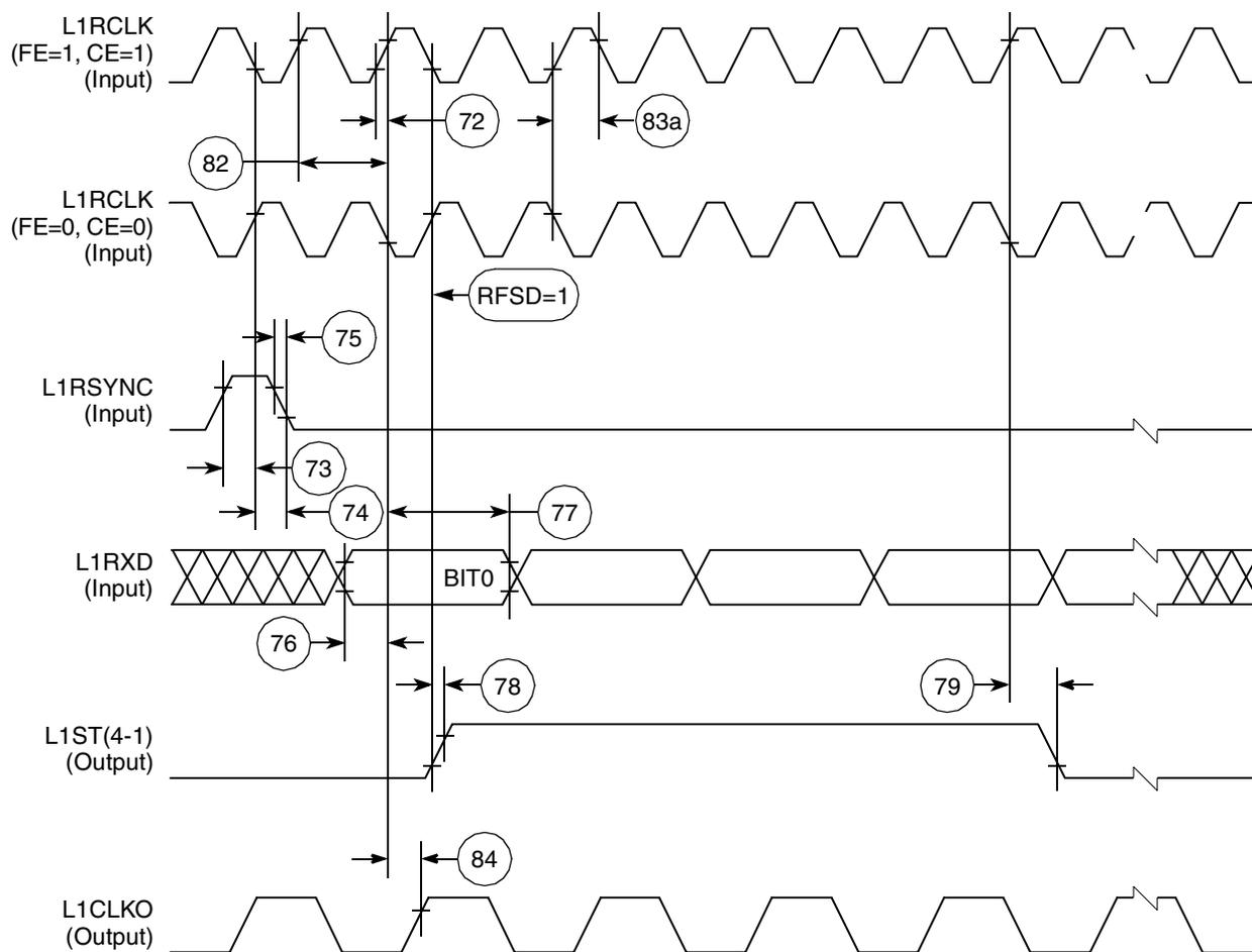
Figure 53. SI Receive Timing with Double-Speed Clocking (DSC = 1)
