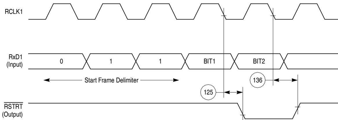
**Figure 63. CAM Interface Receive Start Timing Diagram**
