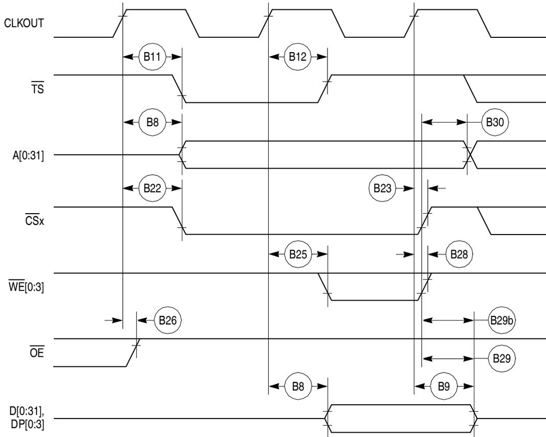
Figure 15. External Bus Write Timing (GPCM Controlled—TRLX = 0,1 CSNT = 0)
