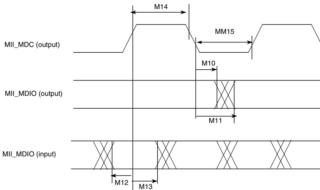
**Figure 76. MII Serial Management Channel Timing Diagram**
