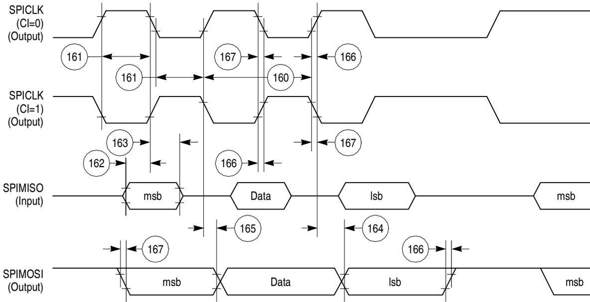
Figure 67. SPI Master (CP = 1) Timing Diagram
