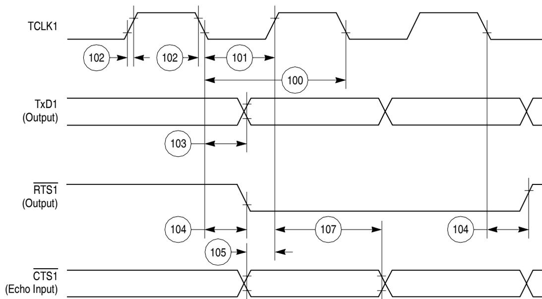
Figure 59. HDLC Bus Timing Diagram
