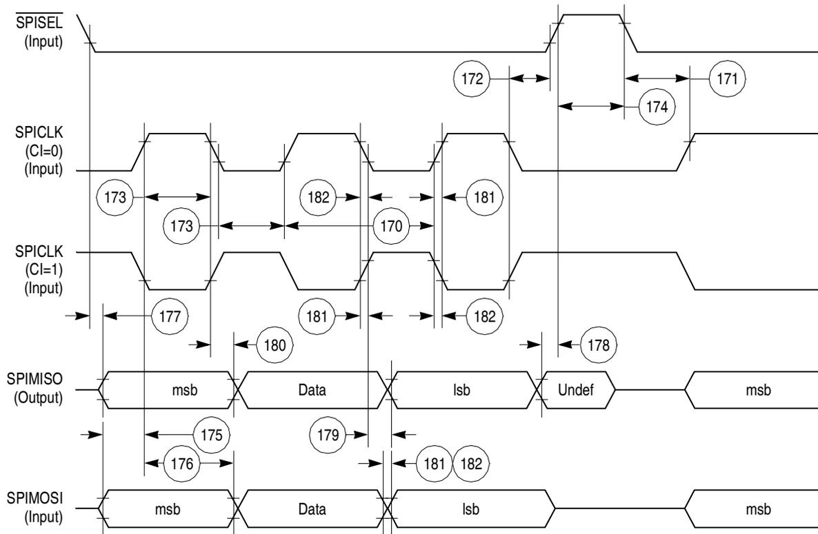
Figure 68. SPI Slave (CP = 0) Timing Diagram
