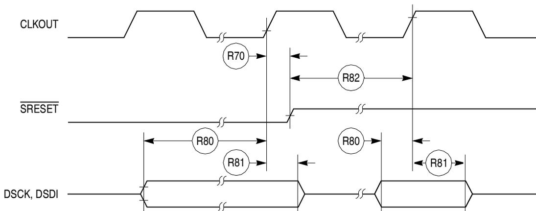
Figure 35. Reset Timing—Debug Port Configuration
