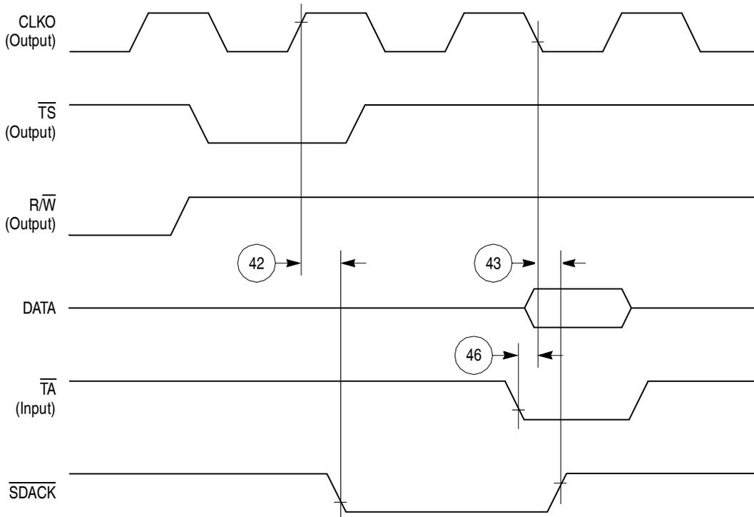
**Figure 47.  $\overline{\text{SDACK}}$  Timing Diagram—Peripheral Write, Externally-Generated  $\overline{\text{TA}}$**
