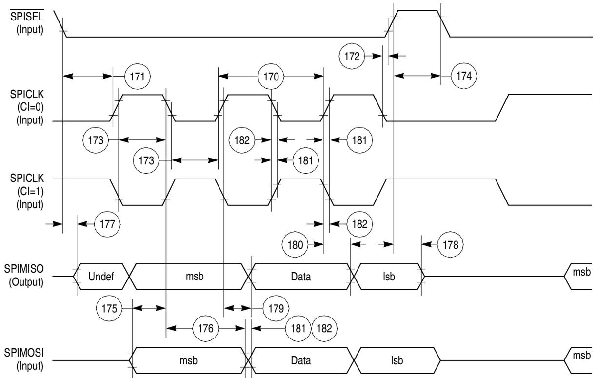
Figure 69. SPI Slave (CP = 1) Timing Diagram
