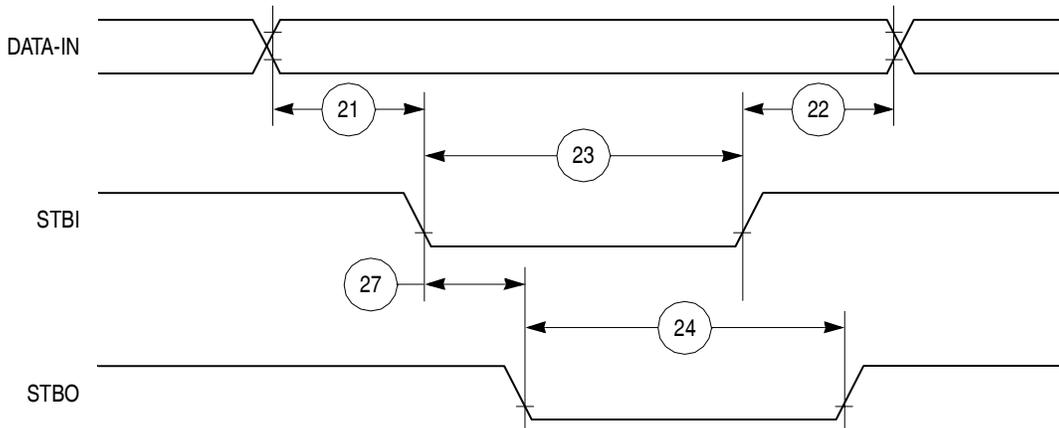
Figure 40. PIP Rx (Interlock Mode) Timing Diagram
