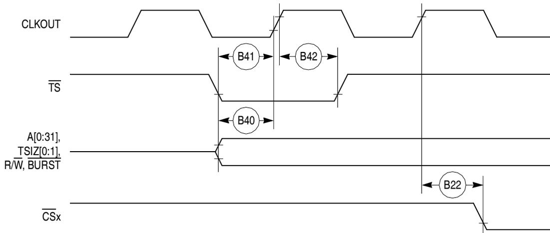
**Figure 21. Synchronous External Master Access Timing
