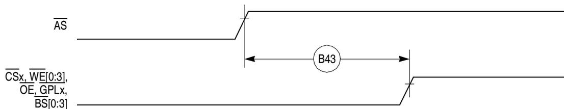
**Figure 23. Asynchronous External Master—Control Signals Negation Timing**
