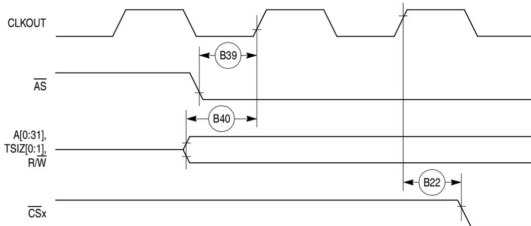
**Figure 22. Asynchronous External Master Memory Access Timing
