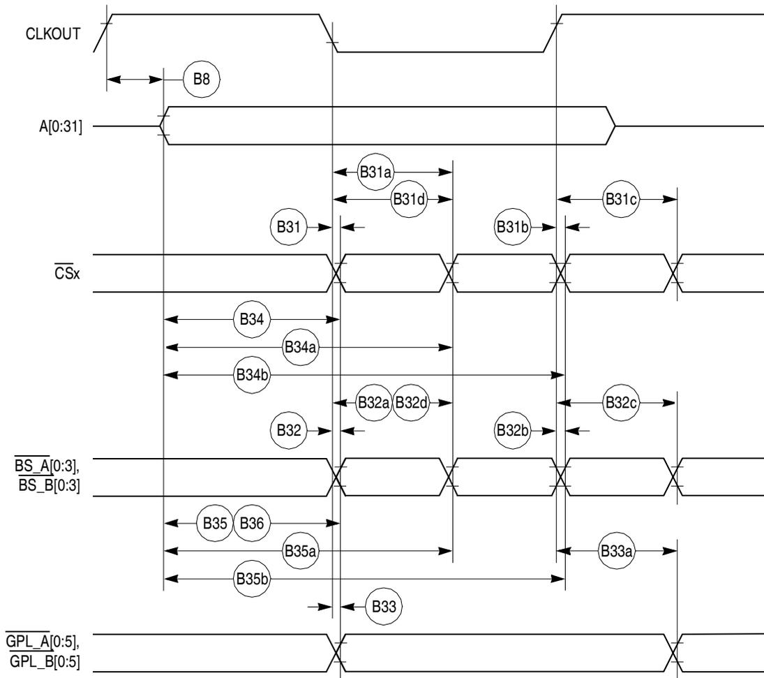
Figure 18. External Bus Timing (UPM Controlled Signals)
