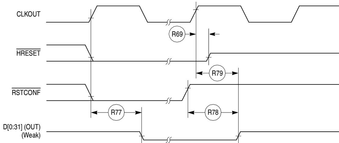
**Figure 34. Reset Timing—Data Bus Weak Drive during Configuration**
