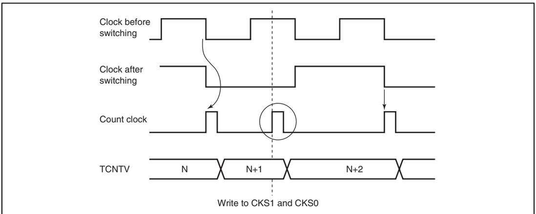
**Figure 10.13 Internal Clock Switching and TCNTV Operation**
