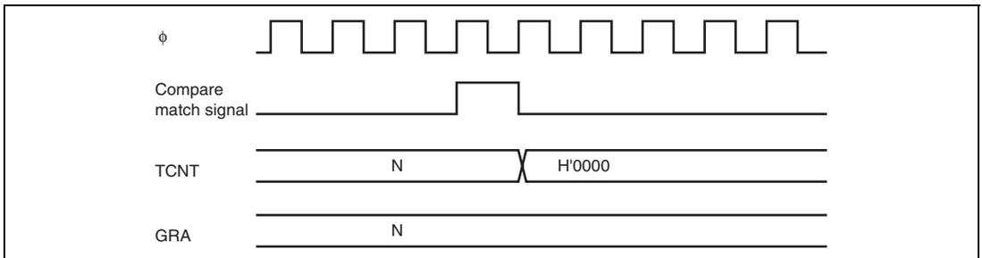
Figure 11.18 Timing of Counter Clearing by Compare Match
