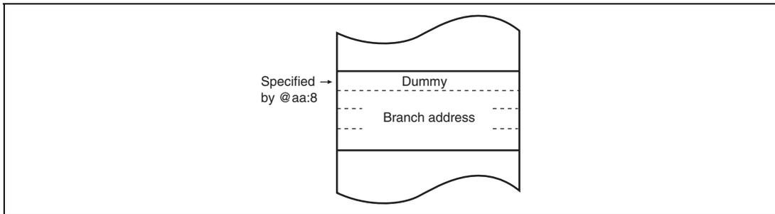
**Figure 2.8 Branch Address Specification in Memory Indirect Mode**
