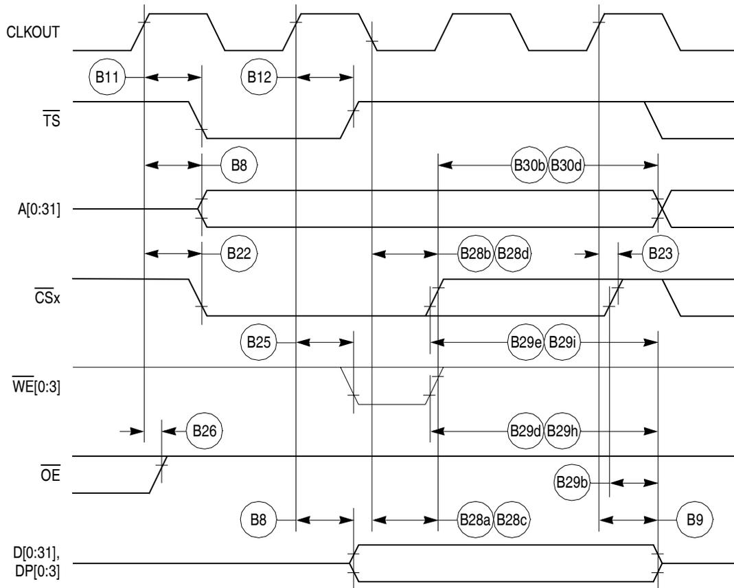
Figure 18. External Bus Write Timing (GPCM Controlled—TRLX = 1, CSNT = 1)
