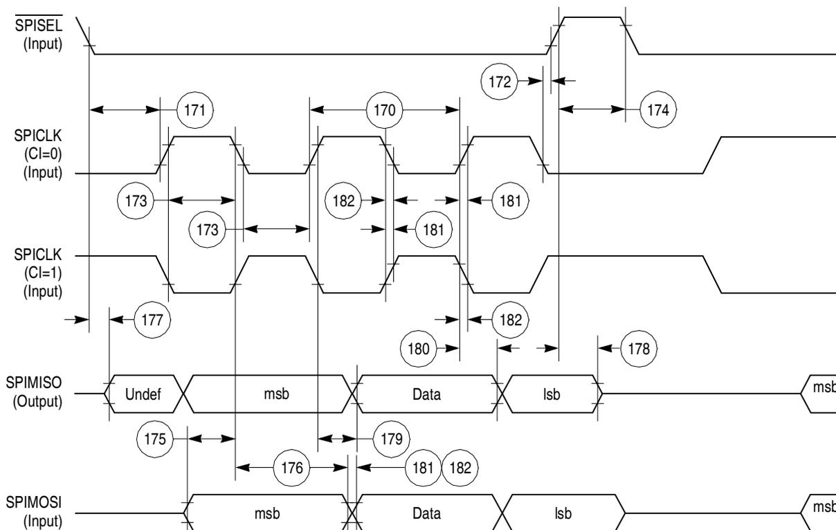
Figure 70. SPI Slave (CP = 1) Timing Diagram
