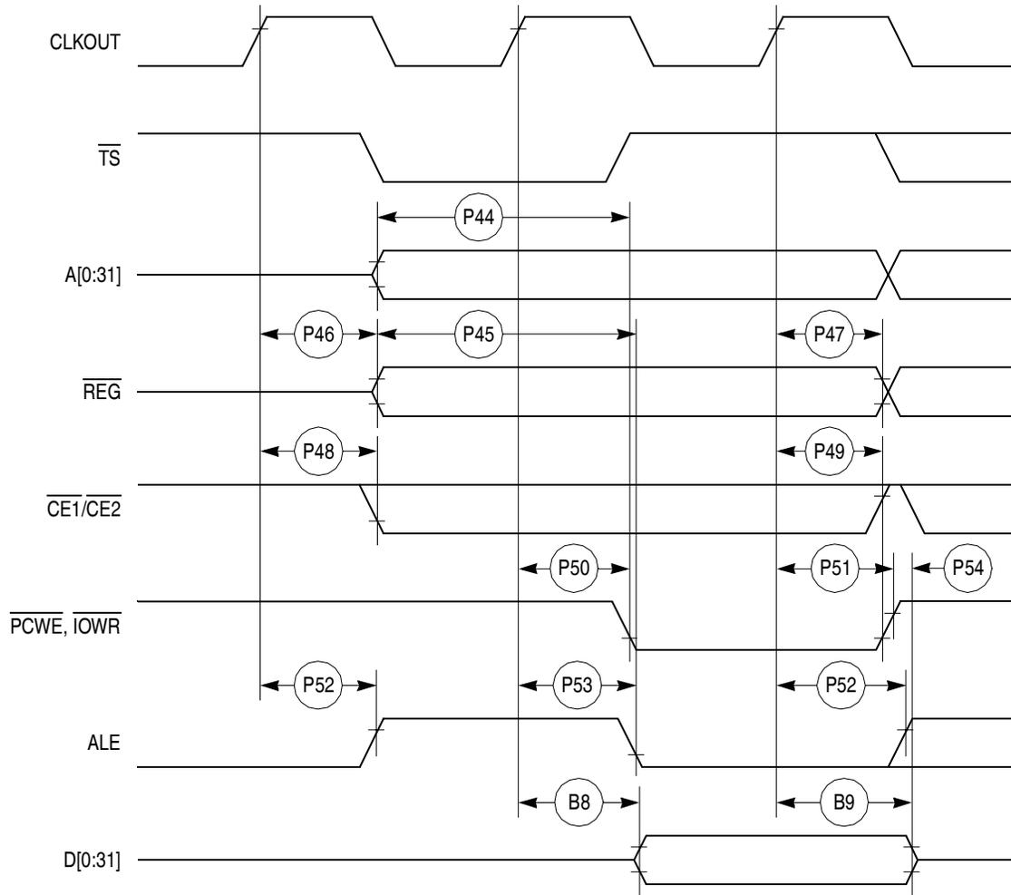
Figure 28. PCMCIA Access Cycles Timing External Bus Write
