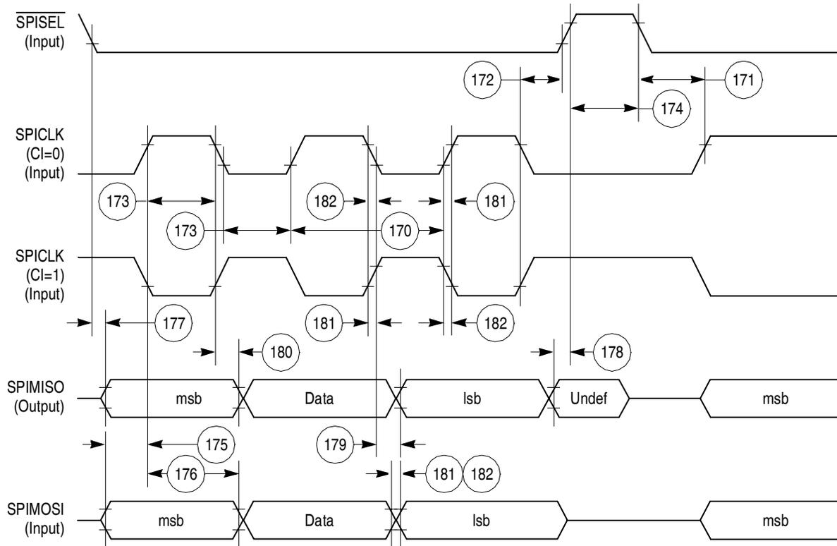
Figure 69. SPI Slave (CP = 0) Timing Diagram
