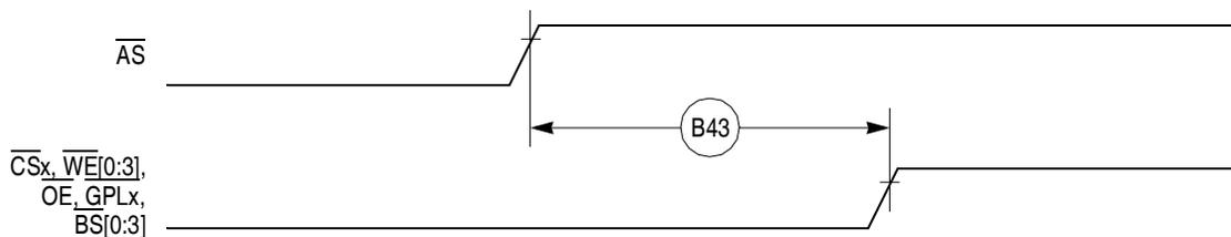
Figure 24. Asynchronous External Master—Control Signals Negation Timing
