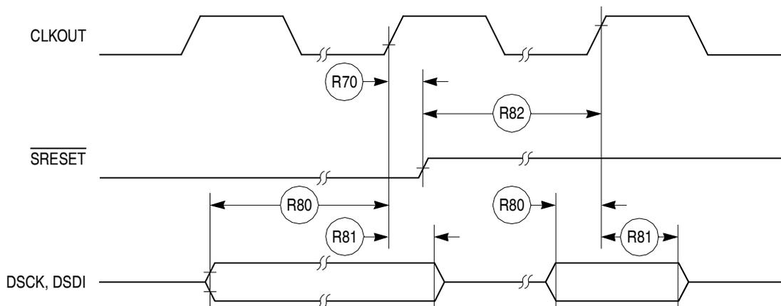
Figure 36. Reset Timing—Debug Port Configuration
