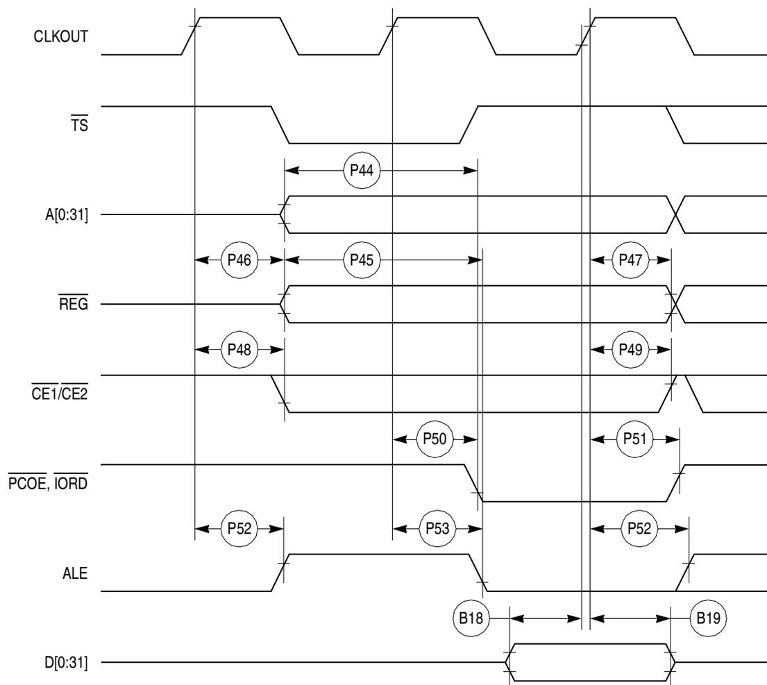
Figure 27. PCMCIA Access Cycles Timing External Bus Read
