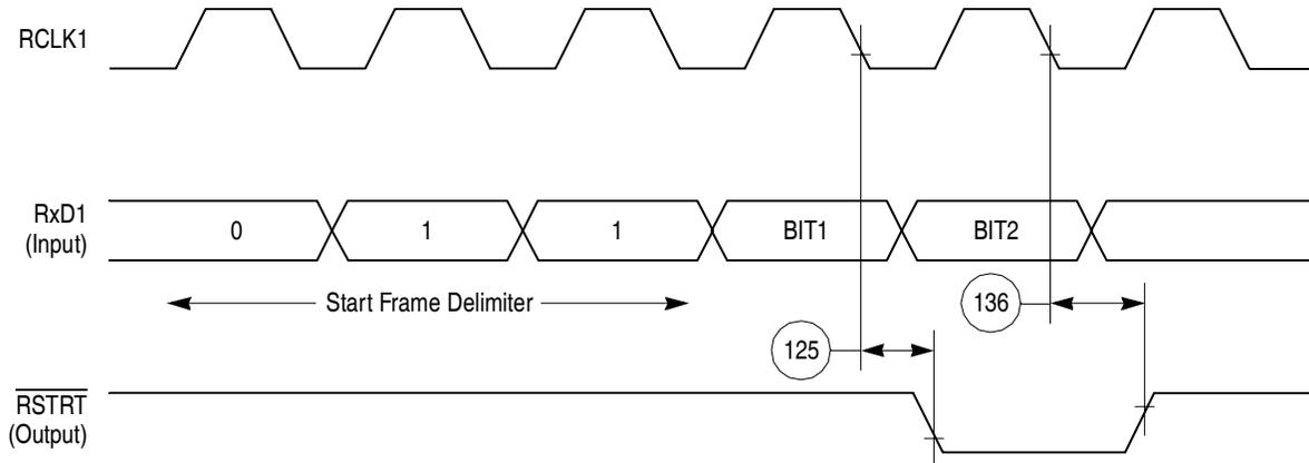
**Figure 64. CAM Interface Receive Start Timing Diagram**
