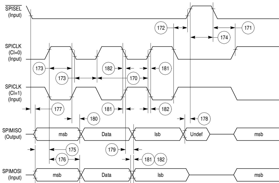
Figure 69. SPI Slave (CP = 0) Timing Diagram
