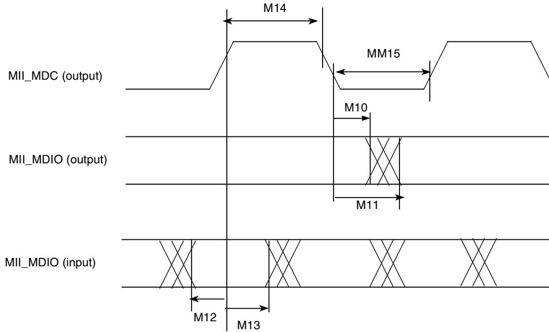
**Figure 77. MII Serial Management Channel Timing Diagram**
