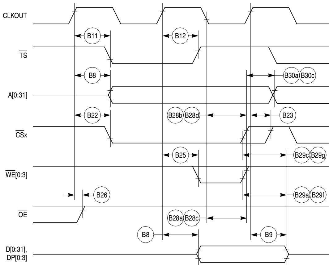
Figure 17. External Bus Write Timing (GPCM Controlled—TRLX = 0, CSNT = 1)
