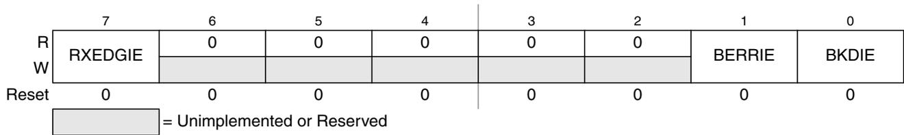
**Figure 10-7. SCI Alternative Control Register 1 (SCIACR1)**
