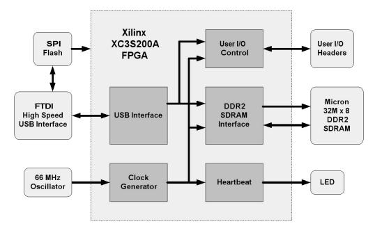
It contains a USB interface block, a User I/0 block, a DDR2 SDRAM interface, a Heartbeat pulse generator, and a clock generator. The SPI Flash is used to store the design's FPGA configuration file.
