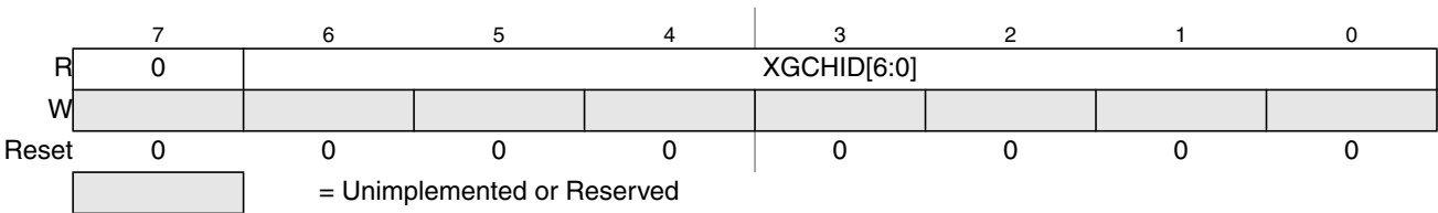
Figure 10-4. XGATE Channel ID Register (XGCHID)
