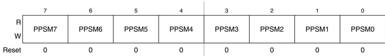
**Figure 2-40. Port M Polarity Select Register (PPSM)**
