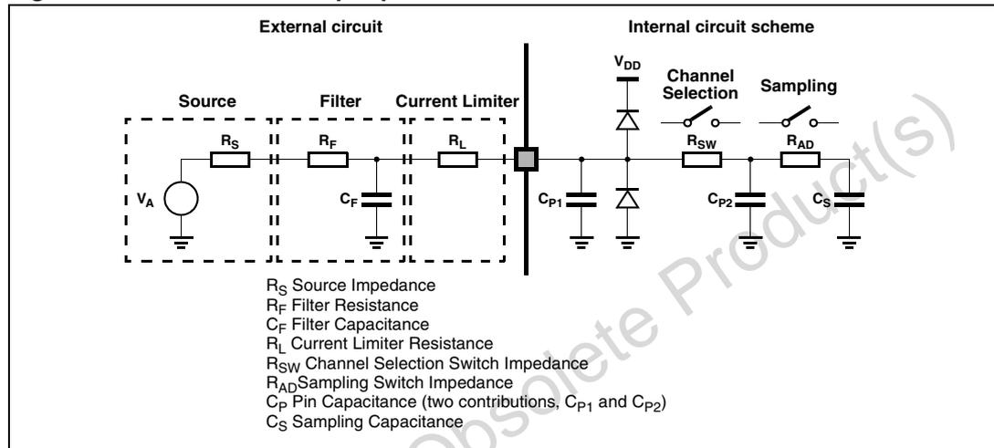
**Input leakage and external circuit**
