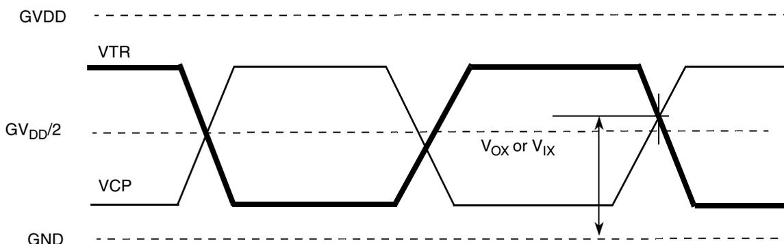
Figure 13. DDR3, and DDR3L SDRAM Differential Timing Specifications
