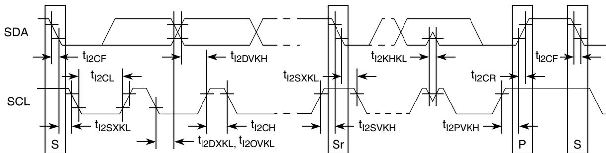
**Figure 31. I<sup>2</sup>C Bus AC Timing Diagram**
