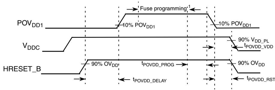
**NOTE:**  $POV_{DD}$  must be stable at 1.5 V prior to initiating fuse programming.
