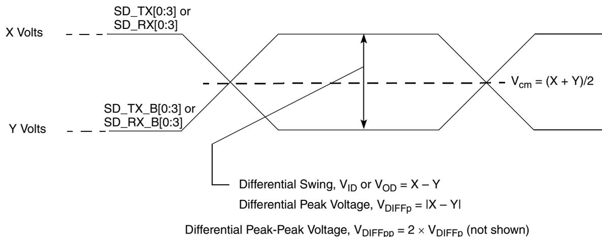
**Figure 36. Differential Voltage Definitions for Transmitter/Receiver**
