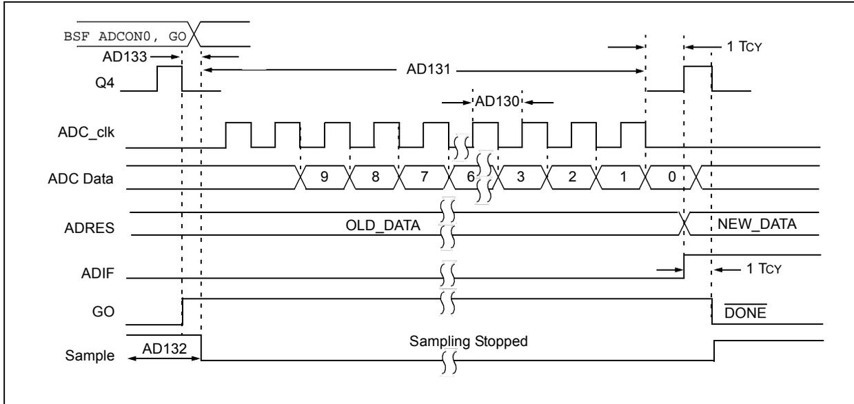
**FIGURE 29-13: ADC CONVERSION TIMING (ADC CLOCK FROM FRC)**
