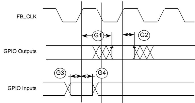
Figure 13. GPIO Timing
