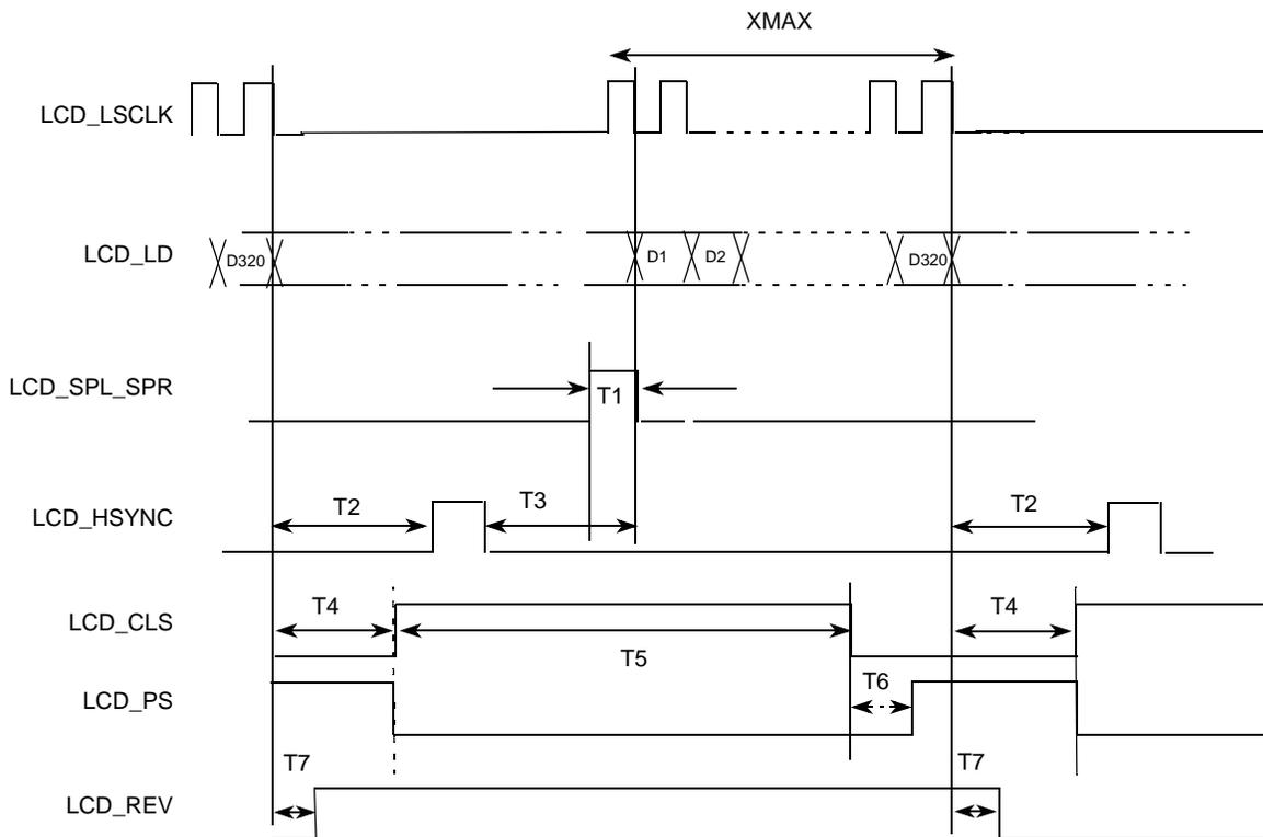
**Figure 17. Sharp TFT Panel Timing**
