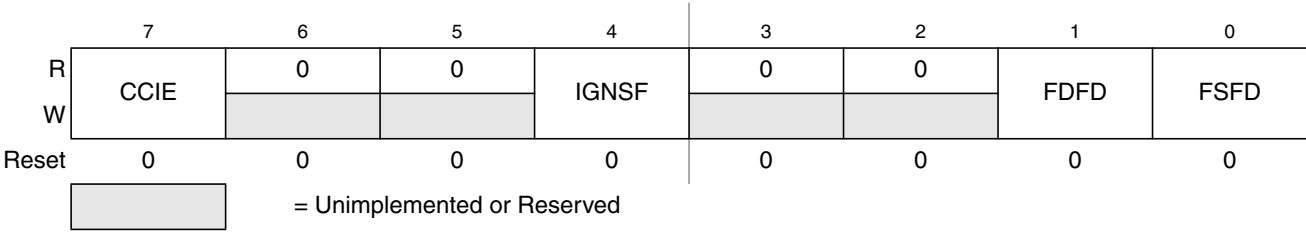
Figure 30-9. Flash Configuration Register (FCNFG)
