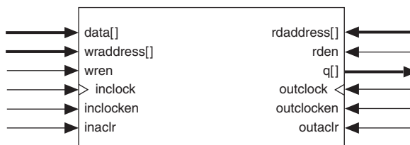
Figure 2–13. Simple Dual-Port and Single-Port Memory Configurations
