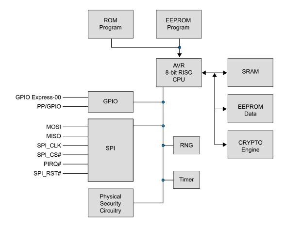
The TPM includes hardware Random Number Generator (RNG), including a FIPS certified Pseudo Random Number Generator that is used for key generation and TCG protocol functions. The RNG is also available to the system to generate random numbers that may be needed during normal operation.
